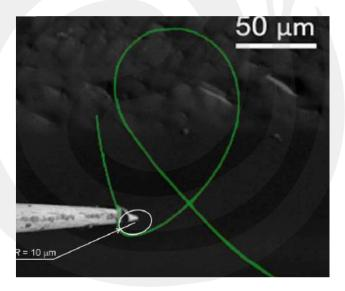
Example of nanofibre obtained by the patented method as can be seen under a scanning electron microscope. The nanofibers are extremely flexible as is shown in the image.
