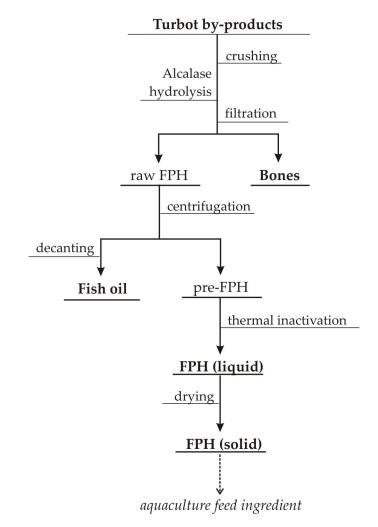
Figure 1. Schematic flowchart of turbot by-products processed through enzymatic hydrolysis.
